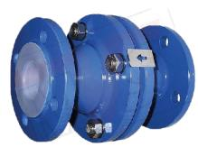
The valve has a Split 2 piece design with FEP / PFA lined ductile iron body and stainless steel fasteners. Its use of FEP and PFA means that it has near universal process corrosion resistance. The valve has a full port developed especially to minimize any pressure loss through the valve.
